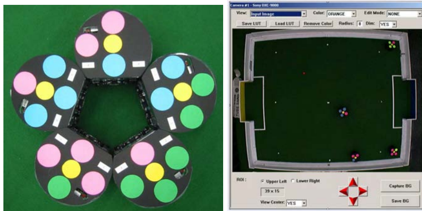
Fig. 5. LEFT: Top view of the 2002 robots. Various color coding schemes were used to make position and orientation determination robust to missed markers. RIGHT: The Vision Calibration GUI. The vision system had to be recalibrated whenever the lighting conditions changed substantially
